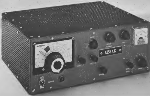
Front view of WA2ELL's and K2SKK's mobile 50-watt transmitter. Unit measures approximately 12 inches in width, 5 inches in height, and 10 inches in depth.
